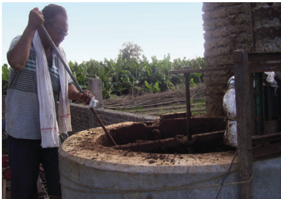
Vijay Ingle stirs the slurry in the biogas digester tank
