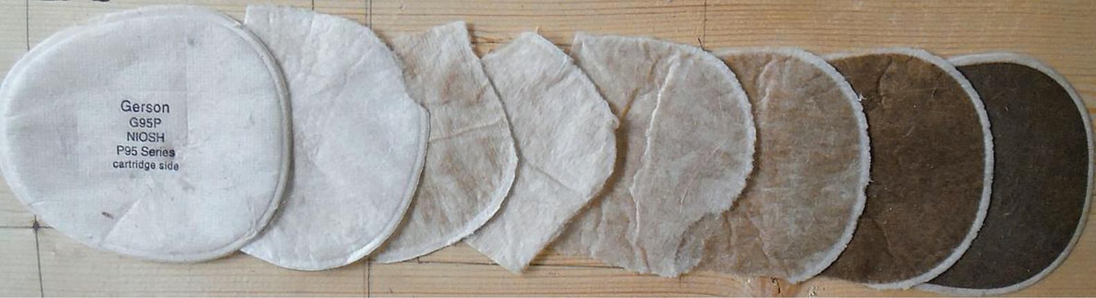
**Cross section of a P95 Mask:** Masks work through multiple layers as depicted above. Each layer further filters out a particular particulate component.
